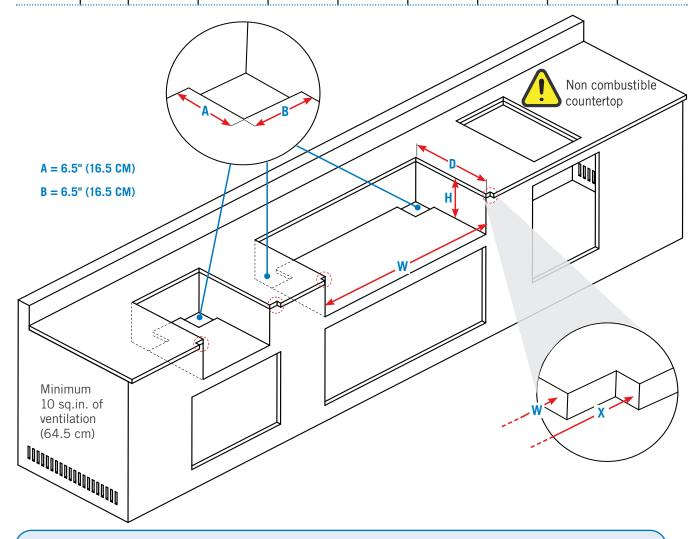
**WARNING!** The cabinet frame, the cabinet and the counter top MUST be made from non-combustible material when the appliance is not installed with the Zero Clearance Liner corresponding to your unit. Refer to the parts list in your Assembly Guide for specific information.
